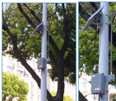
The installed gateway running on solar energy
