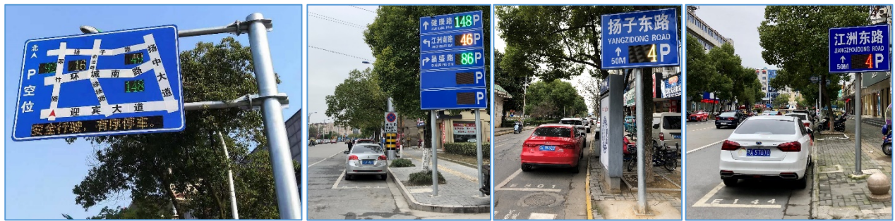
Yangzhong Smart Parking System's intelligent LED traffic guidance signs (1 st level, 2 nd level and two 3 rd level sign) by EPS
